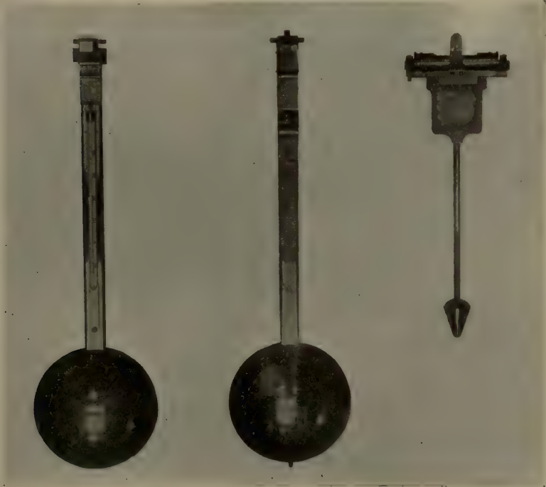
FIG. 85. Dummy Pendulum (with thermometer), Regular Pendulum, and Leveling Pendulum. (C. L. Berger and Sons.)
